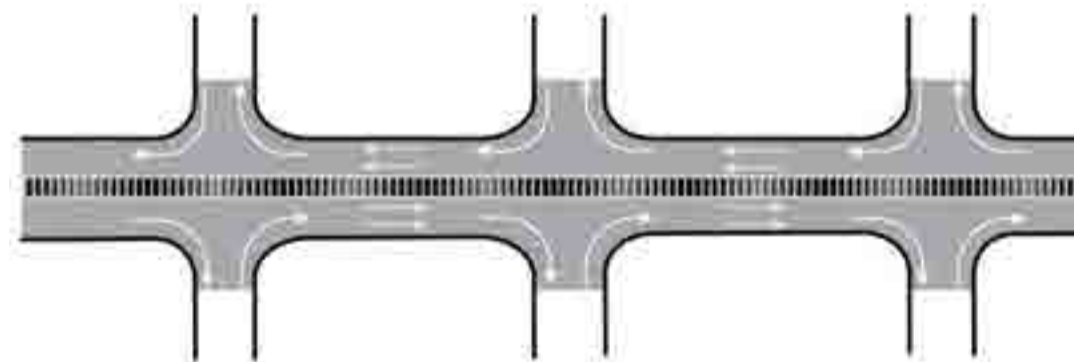
RIGHT-IN/RIGHT OUT WITH RAISED MEDIAN
